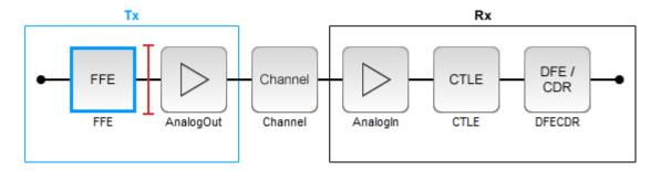
Select the FFE block in the Tx subsystem. In the **Block Parameters** window, change **TapWeights** from  $[0\ 1\ 0\ 0]$  to  $[0\ 1\ 0\ 0]$ , so that the FFE has one pre tap, one main tap, and two post taps. Leave all other blocks in their default settings.
