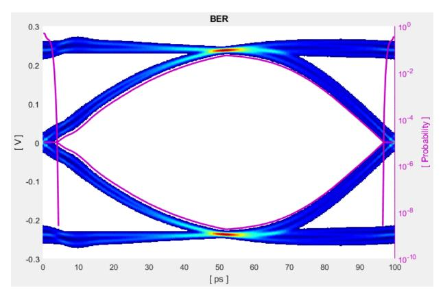
The eye diagram is used to determine the quality of signal integrity. An "open" eye indicates higher probability of bit recovery. The bathtub curve plots the bit error rate as a horizontal function of the data eye, and corresponds to eye-width. The contour curve plots the bit error rate as a vertical function of the data eye, and corresponds to eye-width.
