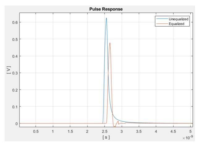
Notice the difference in the pulse response before and after equalization.
